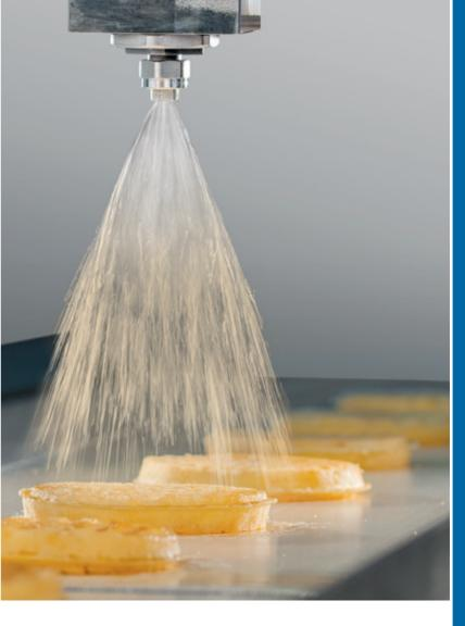
AccuCoat® Spray Systems eliminate the problems often associated with applying coatings such as oils, glazes, release agents and other viscous coatings. Precise heating of viscous coatings ensure that the solution is at the ideal temperature for spraying but not too hot to burn or impact product quality. Cooling of coatings such as egg wash is also possible.
